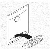
The drip tray for your refrigerator's water dispenser comes from the factory detached. Its removal also allows easy cleaning. To install the drip tray, fit it into the bottom of the dispenser bay and snap into place.
