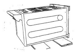
2. Remove the crate wires holding the crate base to the base frame. This can be done with a screwdriver.
