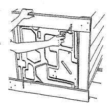
3. Loosen the leveling locking nuts and install the vinyl feet.
