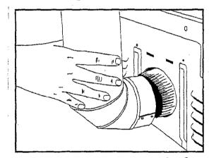
Tip for tight installations: install a section of exhaust system to the dryer before moving the dryer in place. Use duct tape to secure this section to the dryer but do not cover louvers in dryer cabinet.
