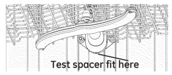
If loose place 2 spacers between the mid conduit and main conduit. If the gap between the conduit and the docking port is large enough to fit 2 spacers stacked on top of each other, proceed to step 2 and use all 4 spacers in step 4.
