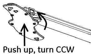
Remove the top screw behind the top spray arm and remove 2 screws securing docking cone to rear tub wall and discard. Carefully pull the top away from the tub (it is not necessary to remove the main conduit).
