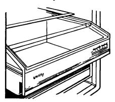
The humidity controls give you the ability to change the amount of moisture in the drawer and/or crisper according to what food you store in them. See the Food Storage Guide on page 18 to determine which humidity setting to use. Move the lever to the right for higher humidity or to the left for lower humidity. The humidity-controlled utility drawer and the crisper are interchangeable. The ClearVue section allows you to see into the drawer/crisper without opening it.
