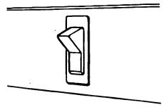
The power on/off switch is located behind the upper ventilation panel. It is used to turn the power to the refrigerator-freezer off when cleaning or changing light bulbs.
