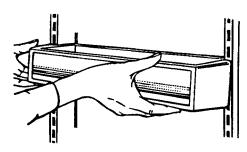
Door bins can hold two-liter bottles and can be placed in any position on the refrigerator door.
