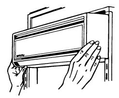
The utility compartment can be placed in any position on the refrigerator door.
