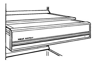
The WinterChill Meat Locker is designed to provide colder storage temperatures than the average refrigerator temperature. The Meat Locker can be located in any set of ladder slots. For temperature controlled use, however, the Meat Locker must be located in one of the six sets of ladder slots starting just below the WinterChill Meat Locker Temperature Control.
