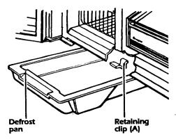
The defrost pan is located behind the base grille toward the left side of the refrigerator-freezer.
