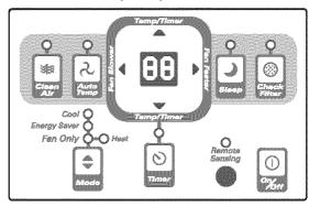
A 2 Digit Display is used to indicate the Fan Speed setting, from 10 through 99. When the "SLOWER" button is pressed the motor speed will slow down at various intervals, down to a minimum setting of 10. To speed the motor up, press the "FASTER" button. The speed will increase at multiple intervals to a maximum setting of 99. Display will revert back to temperature setting after a short time.
