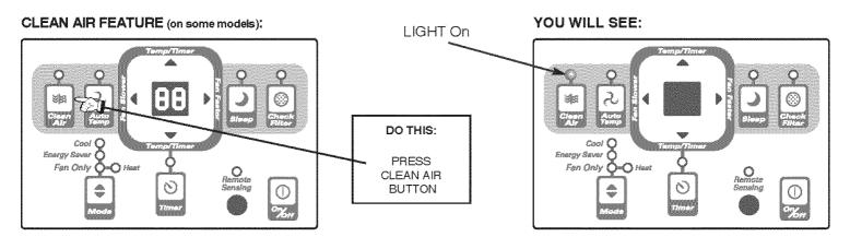
Note: When this feature is "ON", the electronic air purifier is energized to remove pollen and impurities from the air. To cancel this feature,
