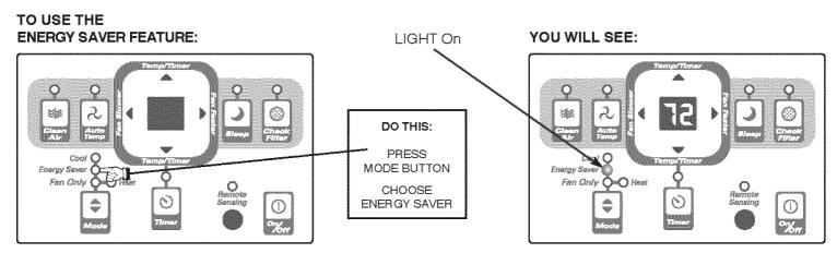
**Note:** In this mode, the fan will continue to run for another 3 minutes after the compressor shuts off. The fan then cycles on for 2 minutes at 10 minute intervals until the room temperature is above the set temperature, at which time the the cooling system turns back on.
