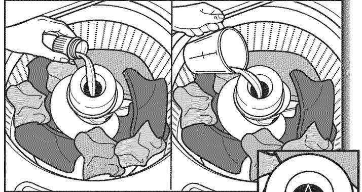
Pour a measured amount of liquid fabric softener into dispenser (on some models); always follow manufacturer's directions for correct amount of fabric softener based on your load size.
