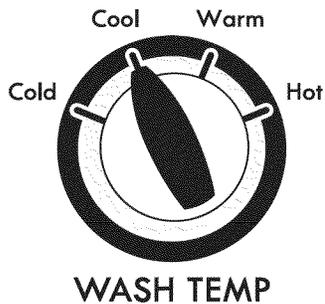
After selecting the load size, select the Wash Temp by turning knob to desired temperature. All rinses are tap cold.
