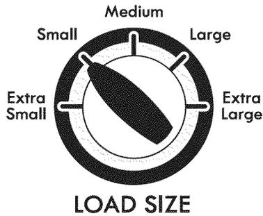
Select the load size setting most suitable for your load. Extra Small will add a low amount of water for smaller loads and Extra Large will add the most amount of water for large or bulky loads. Items need to move freely.
