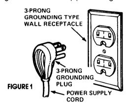
**ELECTRICAL GROUND IS REQUIRED ON THIS AP- PLIANCE.** A 120-Volt, 60 Hz, AC only 15 Ampere fused electrical supply is required. (Time delay fuse or circuit breaker is recommended.) It is recommended that a separate circuit serving only this appliance be provided. DO NOT use an extension cord.
