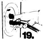
Attach the hose from the hot water faucet to the bottom inlet valve opening (marked "H") on the washer The cold water hose attaches to the top inlet valve opening (marked "C").
