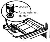
The shutter for the bottom (oven) burner is near the back wall behind the storage drawer or warming drawer. Remove the drawer. See the *Care and cleaning of the range* section.
