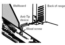
Install the sleeve anchor into the drilled hole and then install the lag bolt through the device. The bolts must be properly tightened as recommended for the hardware.
