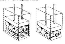
Load bulky trash, bottles, and cans in the center of the drawer. Bottles or cans not placed in the center may become caught between the ram and the drawer. The Drawer Monitor Switch then senses a "misload" and causes the ram to return to the "up" position without compacting.
