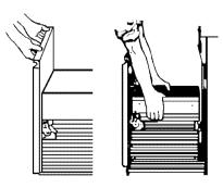
4. Place the other 2 corner posts on the floor to the side of the compactor. Grasp the sides of the compactor cabinet and put compactor on its side on top of the corner posts. Remove the shipping base from the bottom of the compactor.
