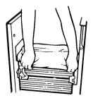
2. Lock bag in place by pulling the four prepunched holes over the bag retainer buttons. Holes will expand over the buttons without damaging the bag. Press inside of bag against the drawer bottom, sides and corners for a smooth fit.
