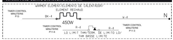
When the Warm and Serve Drawer is first turned on, a "Preheat" circuit is established to provide full power (120 volts). When the temperature at the preheat thermostat reaches 150°F the thermostat opens, and the warmer element starts cycling. If the control is placed on a lower setting, it is possible for the temperature in the drawer to drop enough to allow the preheat thermostat to close again which will allow the element to reenter the "Preheat" mode at full power.
