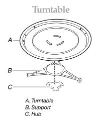
The turntable can rotate in either direction to help cook food more evenly. Do not operate the microwave oven without having the turntable in place. See "Assistance or Service" to reorder any of the parts.
