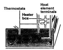
Electric dryer with back panel removed
