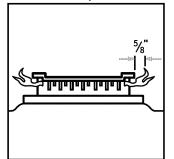
size and shape as shown. A good flame is blue in color. If the flames are uneven, you may need to clean the burner ports.
