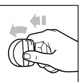
clockwise to the LIGHT position. The clicking sound is the ignitor sparking. Make sure the burner has lit.
