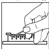
straight pin. Do not enlarge or distort the port. Do not use a wooden toothpick. If the burner needs to be adjusted, call a qualified technician for service. **5.** After cleaning the gas tube opening and ports,
