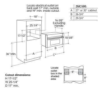
Built-in microwave/convection ovens require a 120 volt, 60Hz power supply. A separate circuit, protected by a time delay fuse or circuit breaker, is required.
