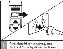
If the Hand Mixer is running, stop the Hand Mixer by sliding the Power switch to the "O" (Off) position. Then, unplug the Hand Mixer from the electrical outlet.
