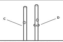
Paired accessories (beaters, optional dough hooks) include one accessory with a collar (D), and one without (C). Single accessories come with a collar (D) (liquid blending rod) or without (C) (whisk).
