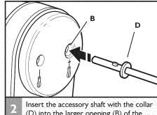
Insert the accessory shaft with the collar (D) into the larger opening (B) of the hand mixer. Align the flanges on the shaft with the slots in the opening. Push to lock into place.
