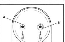
Insert the accessory without a collar (C) into the smaller opening (A). Align and push to lock into place.
