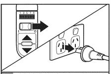
When mixing job is finished, slide the Power switch to the "O" (Off) position. Unplug the Hand Mixer before removing accessories.
