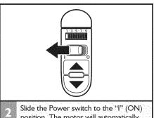
2 Slide the Power switch to the "I" (ON) position. The motor will automatically start at Speed I, and the "I" on the Speed Indicator control will light up.
