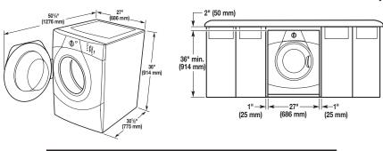
For closet installation, with a door, the minimum ventilation openings in the top and bottom of the door are required. Louvered doors with equivalent air ventilation openings are acceptable.
