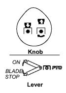
**NOTE:** The PTO knob/lever **must** be in the Blade Stop position when starting the engine, when traveling in reverse and if the operator leaves the seat.
