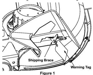
While holding the discharge chute with your left hand, remove the shipping brace with your right hand by grasping it between your thumb and index finger and rotating it clockwise.
