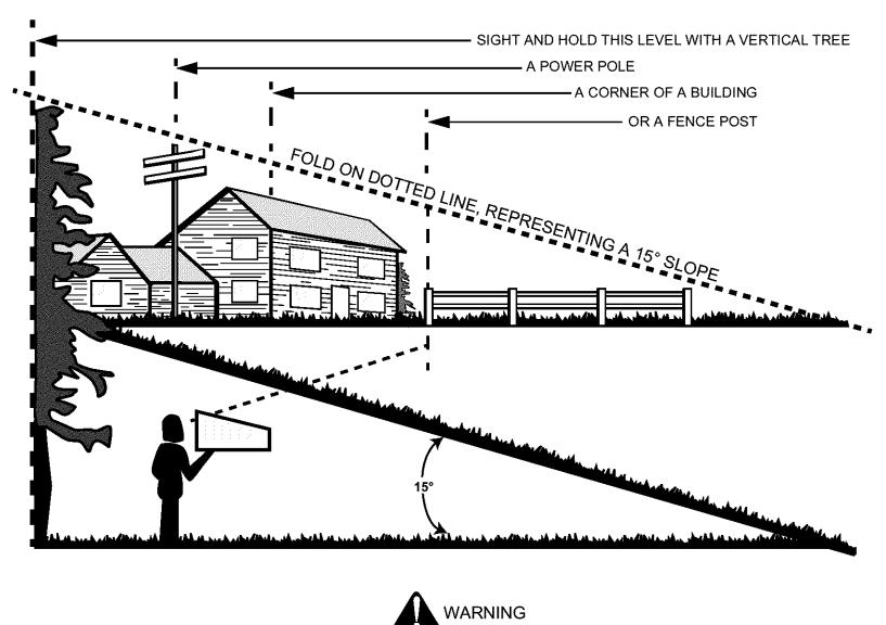
Do not mow on inclines with a slope in excess of 15 degrees (a rise of approximately 2-1/2 feet every 10 feet). A riding mower could overturn and cause serious injury. If operating a walk-behind mower on such a slope, it is extremely difficult to maintain your footing and you could slip, resulting in serious injury.
