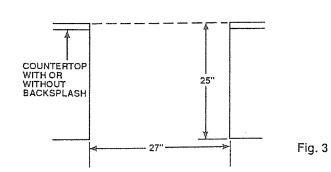
NOTE: If the distance from the back wall to the front of the counter backsplash (Dimension A in Fig. 4) is greater than 1 1/8", there will be a small gap between the wall and the edge of the backguard. This is normal and should not be visually objectionable (See Figs. 3 & 4).
