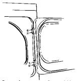
Remove 4 screws—one from each hinge first
