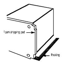
A CAUTION: To prevent damage, do not use the control panel as a means to pick up or move the dryer.
