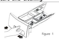
(Lock tab is visible only after drawer has been pulled out)
