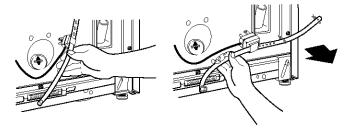
Pull firmly to remove the end of the shipping strap that remains pinned to the back of the washer. This will release the rear self-leveling feet.
