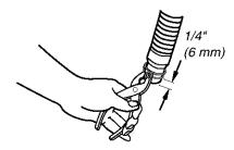
4. Open clamp. Twist hose back and forth while pushing down onto drain connector at the bottom of the washer. Continue until hose contacts the ribbed stop on the cabinet.
