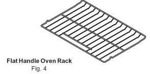
Your range may be equipped with one or more of the oven rack types shown above; a Flat Oven Rack (Fig. 3) or Flat Handle Oven Rack (Fig. 4).
