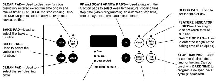
**OVEN, PREHEAT & LOCK LIGHTS**— The "**OVEN**" light will glow each time the oven turns on to maintain the set oven temperature. The "**PREHEAT**" light will glow when the oven is first set to operate, or if the desired temperature is reset higher than the actual oven temperature. The "**DOOR LOCKED**" light will flash when the oven door locks and unlocks or when using the self-clean cycle or the oven door lockout mode is activated. The indicator light will glow constantly after the door locks.
