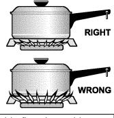
Never extend the flame beyond the outer edge of the utensil. A higher flame simply wastes heat and energy, and increases your risk of being burned by the flame. *For most cooking*, start on the highest control setting and then turn to a lower one to complete the process. Use the recommendations below as a guide for determining proper flame size for various types of cooking. The size and type of utensil used and the amount of food being cooked will influence the setting needed for cooking.
