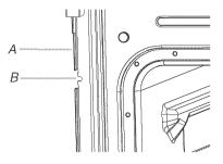
A. Mounting rail B. Insert screw
