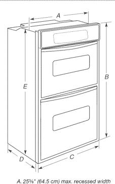
A. 25% (64.5 cm) max. recessed width B. 51" (129.5 cm) max. overall height C. 26¾" (67.9 cm) overall width D. 23" (58.4 cm) max. recessed depth E. 49½" (125.7 cm) recessed height
