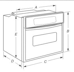
A. 25%" (64.5 cm) max. recessed width B. 29" (73.7 cm) max. overall height C. 26¾" (67.9 cm) overall width
