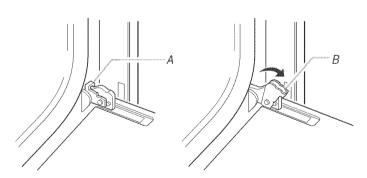
A. Oven door latch in locked position
