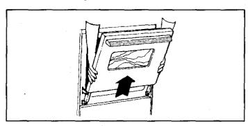
**CAUTION:** Hinge arms are spring mounted and will slam shut against the oven if accidently hit. **Never place hand or fingers between the hinges and the front oven frame.** You could be injured if hinge snaps back.
