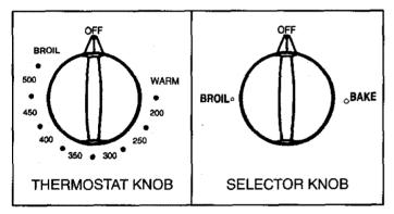
The Selector knob determines the type of oven operation. Turn this knob to the desired setting. Each setting is identified by an indent (stop) and a "click" sound. (Note: The lower oven for double wall oven models does not have a Selector knob.)
