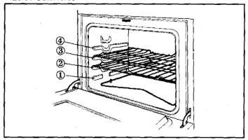
Rack 4 (top of oven) used for two-rack cooking.
