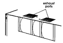
e. Place blower unit back into cabinet. Check that exhaust ports face the top of the cabinet.
