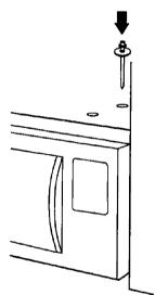
Drop the lock pin and washer assembly into hole "N" and push pin down as far as it will go.
