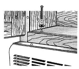
20 ■ Place washers over two, 1/4" x 3" bolts. Then insert a bolt down through each hole in the upper cabinet bottom. Tighten the bolts until the gap between the upper cabinet and microwave oven hood is closed.
