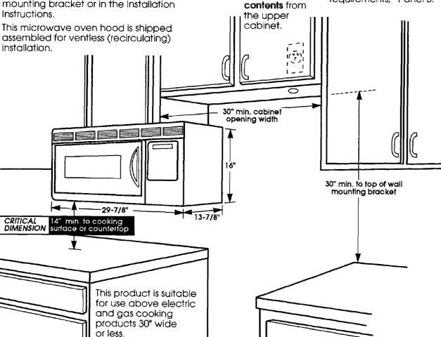
**Wall construction** should be a minimum of 2" x 4" wood studding and 3/8" thickness drywall or plaster/lath.
