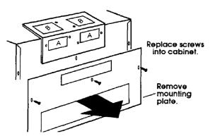
Remove three screws that attach mounting plate to microwave oven hood cabinet. Remove mounting plate and set aside. Replace screws into cabinet.
