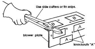
f. Use side cutters or tin snips to cut and remove knockouts marked "A" from blower plate. Discard knockouts.
