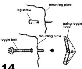
Insert lag screws (wall stud) or toggle bolts (drywall) through the holes on the mounting plate where the mounting plate will be attached to wall stud or drywall at holes "D", "E", "F", "G", "H" and "I".
