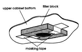
If bottom of upper cabinet is recessed, 2" x 2" filler blocks (not included) the same recess thickness as the upper cabinet will be needed. Mark the center of each filler block and drill a 3/8" diameter hole at the marks. Align filler blocks over the two holes "J" and "K" in the cabinet bottom and attach to cabinet bottom with masking
