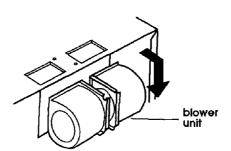
d. Rotate blower unit 1/4 turn (90°) so that the exhaust ports face the top of the cabinet.
