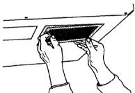
25 Grasp filter screen with one hand holding the ring and the other hand holding the opposite end. Insert the end of the filter screen without ring into the opening and slide towards the center of the microwave oven hood. Insert ring end of filter screen into the opening and slide entire screen towards the side of the microwave oven hood until screen is securely in position. Repeat for other filter screen.
