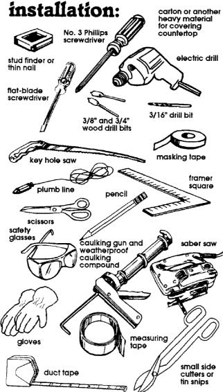
Special hardware and tools are required for brick or masonry walls.
