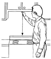
Using a plumb line and measuring tape, determine and clearly mark a vertical centerline on the wall in the area the microwave oven hood is to be installed. Find and mark the location of all wall stud(s) on the wall; then measure and mark their location on the wall template. If there are no wall studs in the area the microwave oven hood is to be installed, consult a local building inspector. Do Not attempt to install microwave oven hood if a wall stud cannot be found.
