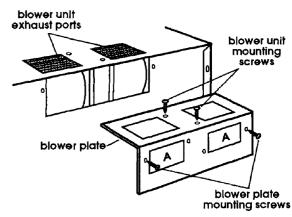
g. Reattach blower plate to cabinet, so exhaust ports and blower plate openings are aligned. Attach with the two blower unit mounting screws and then the two blower plate mounting screws.
