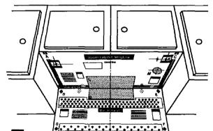
Measure the bottom of the upper cabinet frame. Trim the edges "A", "B" and "C" on the upper cabinet template so that the template will fit on the bottom of the upper cabinet. If upper cabinet has a recessed frame, trim template so that it fits inside the recessed area. Align the centerline of the upper cabinet template with the centerline of the wall template; then securely tape or tack the upper cabinet template in place.
