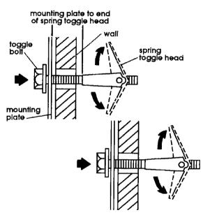
Attach a spring toggle head to the end of each toggle bolt. Leave at least one wall thickness of space between the mounting plate and the end of the spring toggle head so that the spring toggle head can properly open on the other side of the wall.
