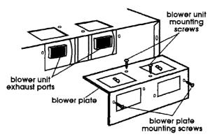
g. Reattach blower plate to cabinet so exhaust ports and blower plate openings are aligned. Attach with the two blower unit mounting screws and then the two blower plate mounting screws.
