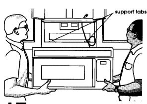
Carefully lift microwave oven hood and hang it on support tabs at the bottom of the mounting plate. Thread power supply cord through the power supply cord hole in the bottom of the upper cabinet.
