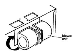
d. Rotate blower unit end over end. Then rotate blower unit 1/2 turn (180°) so that the exhaust ports face the rear of the cabinet. Replace wires into clips at the upper left-hand corner of blower unit.
