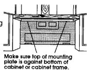
cabinet frame. Start the lag screws through the wall-stud holes and/or insert toggle bolts and spring toggle heads through drywall holes. Tighten screws and/or bolts to secure mounting plate to wall. Check that center of bracket is secured to wall. 16. Slide washer onto lock pin and set inside upper cabinet.
