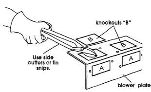
f. Use side cutters or tin snips to cut and remove knockouts marked "B" from blower plate. Discard knockouts.
