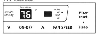
Note: In this mode the selected temperature will increase by 2 °F 30 minutes after the mode is selected. The temperature will then increase by another 2 °F after an additional 30 minutes. This new temperature will be maintained for 7 hours before it returns to the originally selected temperature. This ends the "Sleep" mode and the unit will continue to operate as originally programmed. The "Sleep" mode program can be cancelled at any time during operation by again pressing the "Sleep" button.
