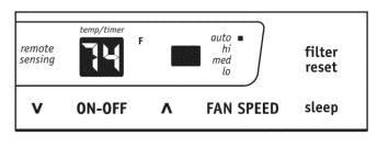
Note: Fan starts at High Speed and adjusts to a slower speeds the room temperature dictates. For example, if the room doesn't get too warm, it will stay at the slowest speed. If the room temperature rises quickly, such as a door being opened, it will automatically go to the highest speed. The fan speeds will re-adjust back to the slowest speed as the room returns to the original set temperature. Press either the fan slower or fan faster button to adjust the fan speed manually.
