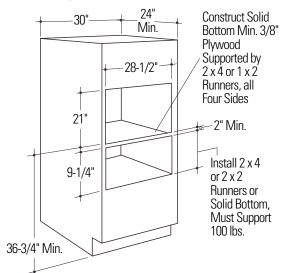
Note: Additional clearance between the cutouts may be required. Check to be sure the oven supports above the Warming Drawer location does not obstruct the required interior 23-1/2" depth and 9-1/4" height. See installation instructions for details.
