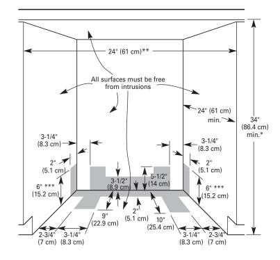
Cut holes in shaded area of cabinet walls or floor as specified below:
