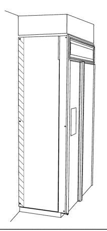
1/4" side panel fitted up to the cabinet trim (top view) on Freezer side.
