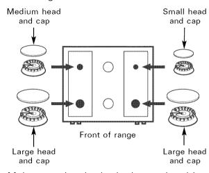
**b**. Make sure the slot in the burner head is positioned over the electrode.
