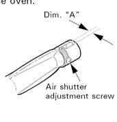
Inner cone of flame ' to 3/4" Oven broiler burner
