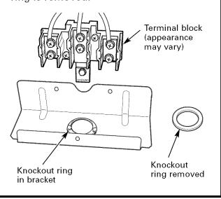
C For power cord installations only (see the next step if using conduit), assemble the strain relief in the hole. Insert the power cord through the strain relief and tighten. Allow enough slack to easily attach the cord terminals to the terminal block. If tabs are present at the end of the winged strain relief, they can be removed for better fit.
