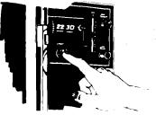
6. Push the START Button. The oven light will stay on You will hear a fan runrung during oven operation.
