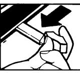
**DO NOT** force the Lock Lever. The lever is designed to stay locked until the oven is cool enough to safely open
