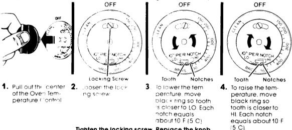
Tighten the locking screw. Replace the knob.
