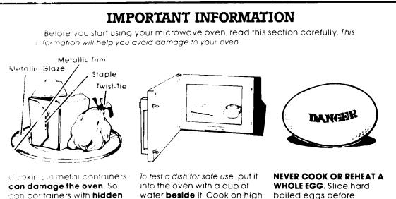
can containers with hidden metal ("wist-ties" foil-lining, staples metallic glaze or trim) Test dinnerware or cook ware before using To test a dish for safe use, put it into the oven with a cup of water **beside** it. Cook on high Cook Power for one minute. If the dish gets hot and the water stays cool, do not use it.
