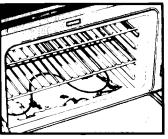
**DO NOT** use foil or other liners in the oven. During the cleaning cycle, foil can burn or melt.
