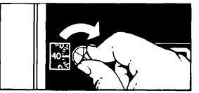
1. Without pushing in the Minute Timer Knob, turn it until the time showing in the window is longer than you want
