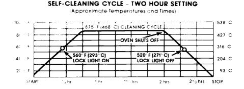
Notice that the heating stops where the two hour setting is up, but that it takes a while Linger for the oven to cool down enough to unlock.
