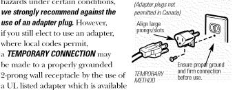
The larger slot in the adapter must be aligned with the larger slot in the wall receptacle to provide proper polarity in the connection of the power cord.
