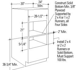
Note: Additional clearance between the cutouts may be required. Check to be sure the oven supports above the Warming Drawer location does not obstruct the required interior 23-1/2" depth and 9-1/4" height. See installation instructions for details.
