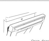
Open door to the "Broil Stop" position when broiling.
