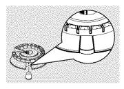
Replace the matching size caps onto the heads. There is one small, two medium and one large cap. Sizes are stamped into the bottom of the caps.
