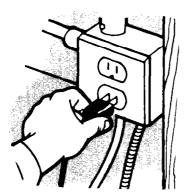
Is the power supply cord plugged into a live circuit with the proper voltage?
