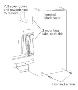
Depending on your electrical supply, make the four-wire or three-wire connection to the range following the "Power supply cord method" or "Direct wire method" instructions for copper wire or aluminum wire depending on the connection needed.
