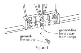
8. Connect the green ground wire from power supply cord to the range using the ground-link screw. The ground wire must be attached first and must not contact any other terminal. See Figure 2.
