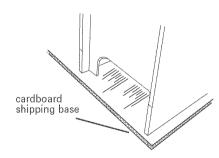
Remove storage drawer. Use a 3/8" drive ratchet to lower rear leveling legs one-half turn. Use channel lock pliers to lower front leveling legs one-half turn.
