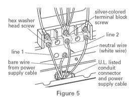
9. Loosen (do not remove) the hex washer head screw and insert the neutral (white) wire under the screw clamp at the bottom of the center position terminal connector. Insert the other two wires (lines 1 and 2) under the other two screw clamps. Securely tighten the hex washer head screws to 90 in/lbs minimum torque to make proper electrical connection. See Figure 5.
