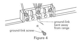
Connect the bare ground wire to the range using the ground-link screw and cup washer. The ground wire must be attached first and must not contact any other terminal. See Figure 5.
