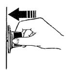
Push in and turn the lower oven drawer knob to any desired setting
