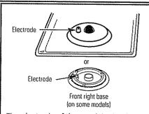
The electrode of the spark igniter is exposed when the burner head is removed. When one burner is turned to LITE, all the burners spark. Do not attempt to disassemble or clean around any burner while another burner is on. An electric shock may result, which could cause you to knock over hot cookware.
