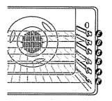
When convection baking with only I rack follow the rack positions recommended in the Using the oven section
