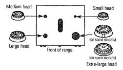
Make sure the slot or hole (depending on model) in the burner head is positioned over the electrode
