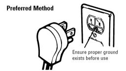
The power cord of this appliance is equipped with a 3-prong (grounding) plug which mates with a standard 3-prong grounding wall receptacle to minimize the possibility of electric shock hazard from this appliance.
