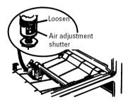
The shutter for the bottom (oven) burner is near the back wall behind the warming drawer. Remove the drawer. See the *Care and cleaning of the range* section.
