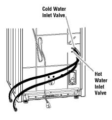
STEP 3. Attach the hose with the blue coupling to the cold water (top) inlet valve. Screw on coupling by hand. Make an additional two-thirds turn with pliers to tighten coupling. DO NOT OVER-TIGHTEN; this could damage valves.
