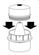
**STEP 7.** Replace the dispenser on the agitator; press firmly to snap into place.
