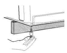
**STEP 4.** Tilt washer backward until front of washer is off the wood block. Remove wood block. Gently lower washer to floor.
