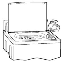
After loading the washer, pour measured liquid chlorine bleach carefully into the dispenser.
