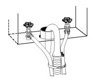
If the water faucets and drain standpipe are recessed, put hooked end of drain hose in standpipe. Tightly wrap the shipping strap around the drain hose and water inlet hoses (not the handles or stems). Push fastener into the nearest hole in the shipping strap.
