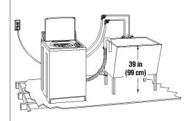
Standpipe Drain System (p. 13)
