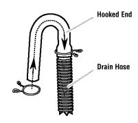
**STEP 3.** Put hooked end of drain hose into laundry tub or standpipe. Check for proper length of drain hose. Rotate hook to eliminate kinks.
