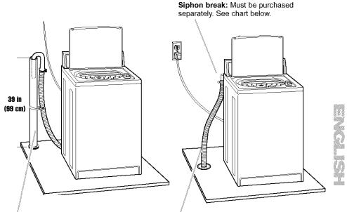
Standpipe drain system: Needs a 2 in (5 cm) minimum diameter standpipe with minimum carry-away capacity of 17 gal (64 L) per minute. Top of standpipe must be at least 39 in (99 cm) inches above floor and no higher than 96 in (2.4 m) from bottom of washer.
