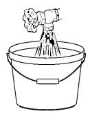
STEP 2. Attach the hose with the red coupling to the hot water faucet. Screw on coupling by hand. Make an additional two-thirds turn with pliers to tighten coupling. DO NOT OVERTIGHTEN; this could damage the coupling.
