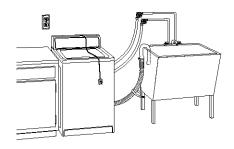
STEP 2. Locate the remaining piece of shipping strap (not the end with the cotter pins) from STEP 3 of "REMOVE SHIPPING STRAP." Use it to wrap the drain hose together with the laundry tub or standpipe. Push fastener into the nearest hole in the shipping strap.
