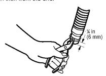
c. Open clamp. Twist hose back and forth while pushing down onto drain connector at the bottom of the washer. Continue until hose contacts the ribbed stop on the cabinet.
