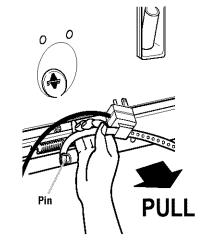
STEP 3. Cut the shipping strap about 16 inches (40 cm) from plug end. Look for the words "CUT HERE." Discard end with the cotter pins. Slide remainder of shipping strap free from the electrical plug. You will use this to secure the drain hose.
