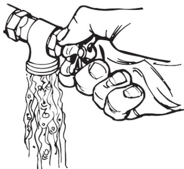
Run water through both faucets into a bucket to get rid of particles in the water lines that might clog hoses. Mark the hot water faucet.
