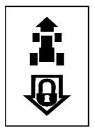
tractor to remain at that speed without applying pressure to the drive pedal. Depress the brake pedal or the drive pedal to deactivate cruise control. Refer to **Setting the Cruise Control** on page 14 this manual for detailed instructions regarding the cruise control feature.
