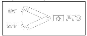
On models equipped with a manual PTO, the PTO lever is located on the left side of the dashboard next to the steering wheel. Move the PTO lever forward to engage the power to the cutting deck or other (separately available) attachments; move the PTO lever rearward to disengage the power to the attachments.
