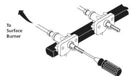
Test to verify if "LOW" setting should be adjusted
