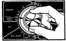
**B.** Stop on a number in the cycle you want. The numbers are minutes of wash time. The drawing shows 10 minutes of agitation in the REGULAR Cycle.
