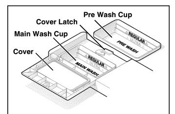
Note: If the cover is closed on the Main Wash Cup, open by pressing the cover latch.
