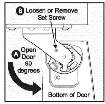
Loosen/Remove Set Screw
