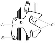
A. Hinge hanger B. Door frame hinge C. Support pins
