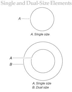
The Dual-Size Elements offer flexibility depending on the size of the cookware. Single size can be used in the same way as a regular element. The dual size combines both the single and outer element and is recommended for larger size cookware, large quantities of food and home canning.
