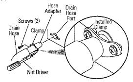
Push plastic conical end of drain hose adapter into washer drain hose port. Insert two screws found in installation pack, and drive screws to mount drain hose to washer.
