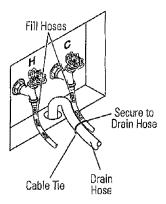
**NOTE:** Drain hose nozzle may be shortened if original length prevents full insertion into drain facility.
