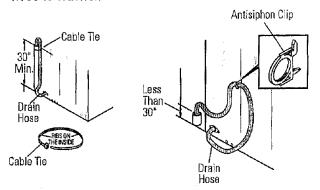
**NOTE:** If drain hose facility does not meet the 30° minimum standpipe height requirement, thread drain hose through supplied antisiphon clip and mount to cabinet back as shown. Mount antisiphon clip by inserting top clip into top mounting hole and snap second clip into position.
